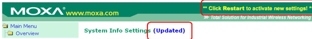
To make the changes effective, click **Restart** and then **Save and Restart** after you change the settings. About 30 seconds are needed for the AWK-6232 to complete its restart process.
