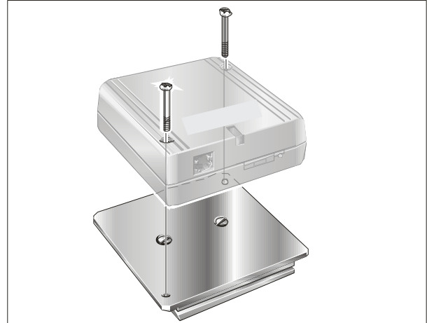
Figure 12: Attaching TC35i Terminal to a top-hat rail
